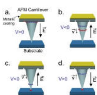
Figure 1. Scheme of operation for mobility measurements using a modified AFM probe
