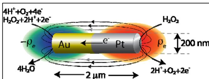
Electrokinetic locomotion is due to reaction induced charge electrophoresis. Dipolar regions of charge density are generated from asymmetric electrochemical reactions of hydrogen peroxide on a bimetallic Janus nanoparticle. Locomotion results from electrical body forces in the surrounding fluid, which are generated by a coupling of an asymmetric dipolar charge density distribution and the electric field it generates.
