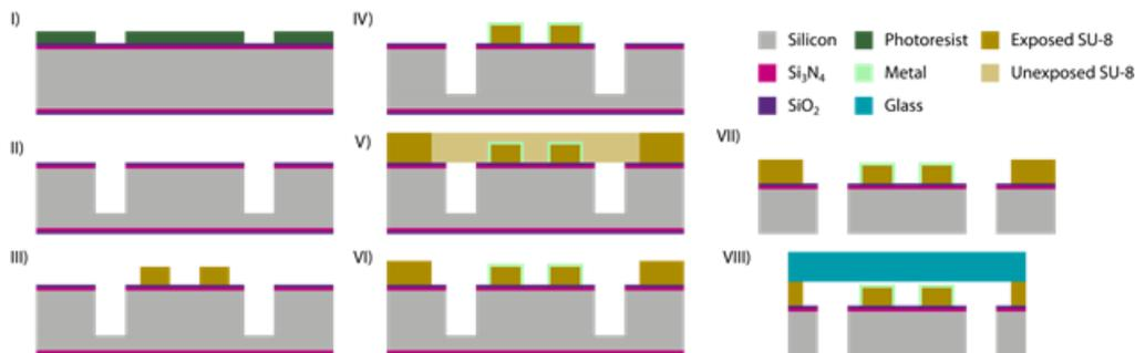
Figure 2: Fabrication process of the electrorotation chips with 3D electrodes
