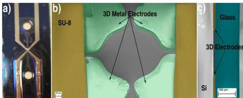
Figure 3: (a) Electrorotation chip; (b) SEM of the 3D metal electrodes; (c) SEM of the cross-section of a chip with the glass coverage.
