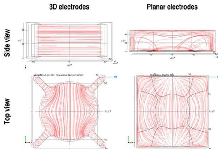
Figure 1: Comsol simulations of the electric field for planar and 3D electrodes
