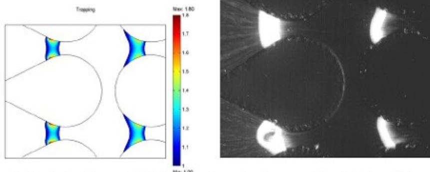
Figure 2. (a) Prediction of the zones for dielectrophoretic trapping when a potential of 500 V is applied with a suspending medium with conductivity of 100  $\mu\text{S}/\text{cm}$  and pH of 8, employing particles having a diameter of 1  $\mu\text{m}$ , (b) Experimental results obtained under the same conditions.
