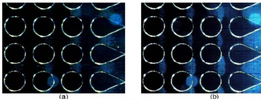
Figure 2. Pictures showing dielectrophoretic microalgae concentration inside a microchannel with cylindrical insulating structures, post diameter is 200  $\mu\text{m}$ , flow direction is from right to left. a)  $E=800$  V/cm; b)  $E=1000$  V/cm.
