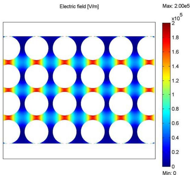
Figure. 1 Electric field distribution across the post array when a 500 V electric potential was applied in a medium with a conductivity of 100  $\mu\text{S}/\text{cm}$  and a pH of 8.
