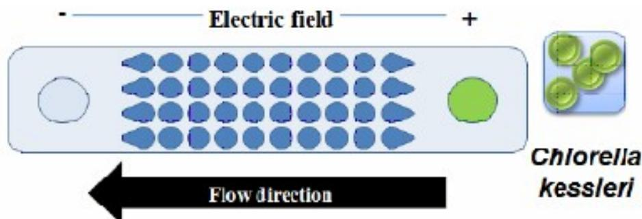
Figure 1. Schematic representation of the microchannel employed for microalgae dielectrophoretic trapping.
