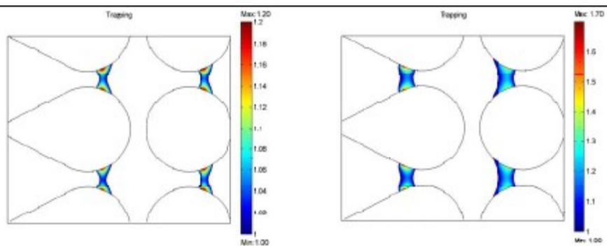
Figure 3. (a) Prediction of the zones for dielectrophoretic trapping when a potential of 600 V is applied with a suspending medium with conductivity of 25  $\mu\text{S}/\text{cm}$  and pH of 8, employing particles having a diameter of 1  $\mu\text{m}$ , (b) prediction of the zones for dielectrophoretic trapping when a potential of 500 V is applied with a suspending medium with conductivity of 100  $\mu\text{S}/\text{cm}$  and pH of 9, employing particles having a diameter of 1  $\mu\text{m}$
